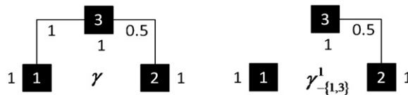
Fig. 7. Deleting the capacity of a link in a fuzzy graph.
